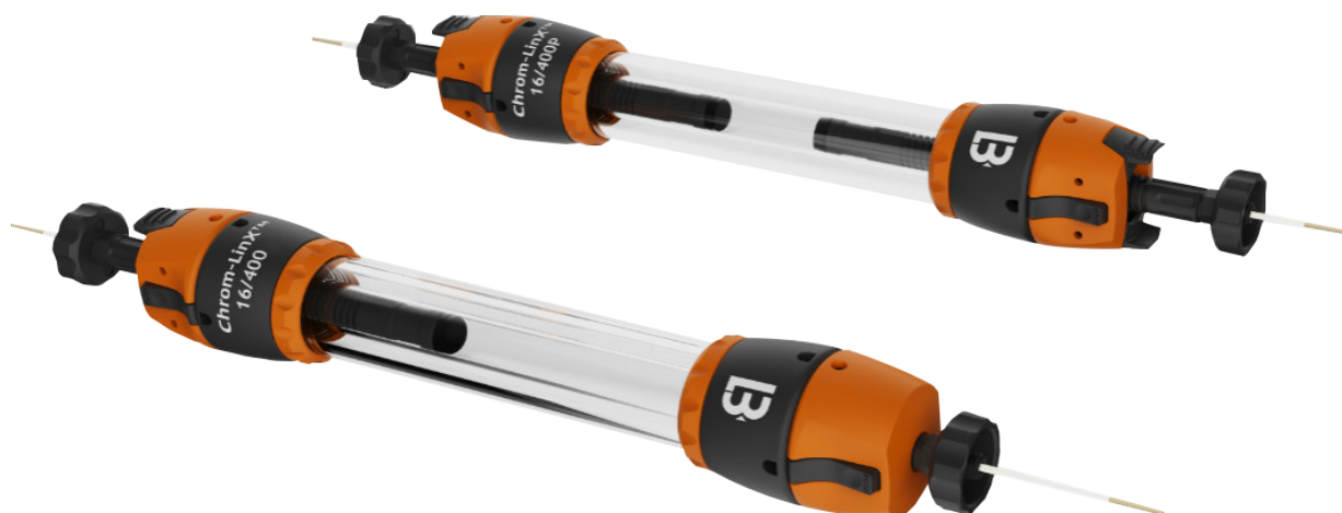
Fig 1. Chrom-LinX® laboratory grade empty chromatography columns
